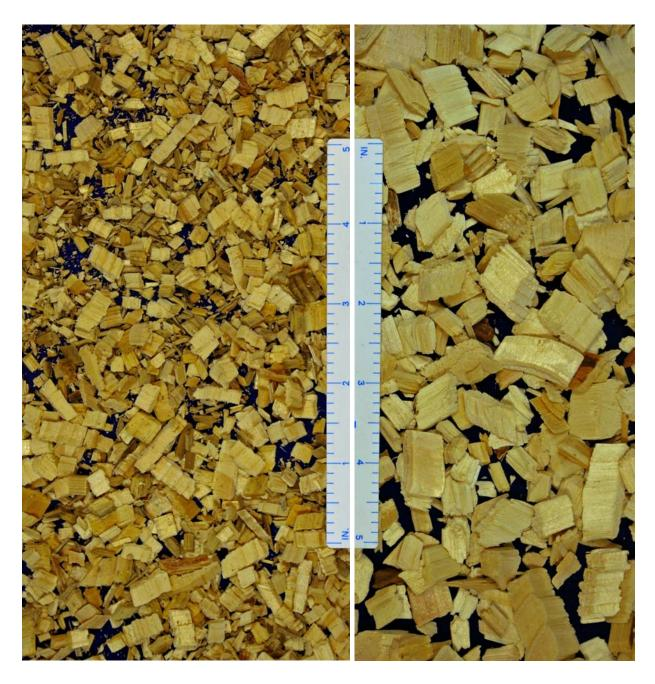
The above photos compare the chips produces with a  $\frac{1}{4}$ " chip length with those produced by a production chipper running a  $\frac{3}{8}$ " chip length and worn anvil. The chips produced by both chip lengths were consistently thin and maintained roughly the same thickness to length ratio that is typically found in larger pulp chips produced by a disc chipper.
