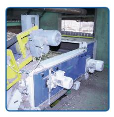
The eddy current separator type 0429 nearly has identical dimensions like the eddy current type 0428 with concentric rotor systmes. This ensures high flexibility regarding the rotor system during all project phases.
